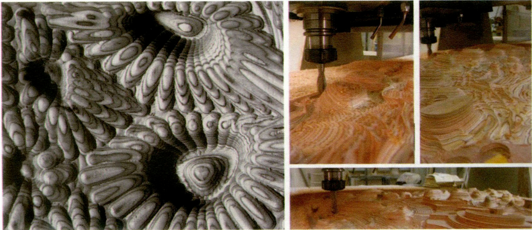
3_Details of machining effects and diversity realized through digital craft protocols. Tools: Rhino, Grasshopper. CNC. Trevor Jordan, Brian Turcza, Austin Weller, and Yoon Jin Kim; Instructor: Brian Ringley
