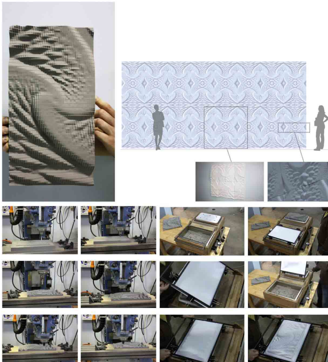
Figure 4: Fabrication process of Fractal Imprint project. The 3D voxel form was controlled by a 2D fractal image.
