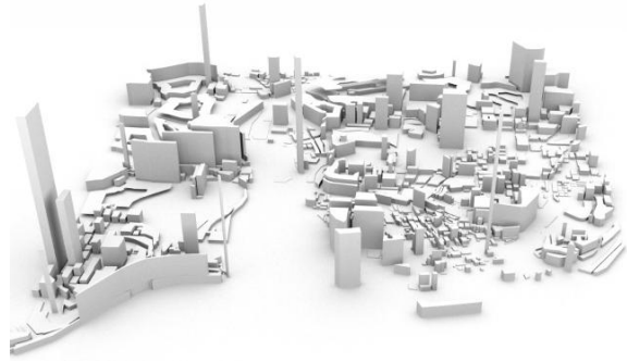
Figure 1: In order to integrate population density into parametric modeling tools so as to construct an urban model parametrically, the population density is visualized by the height of each block. Created by student Jesse Larkins.
