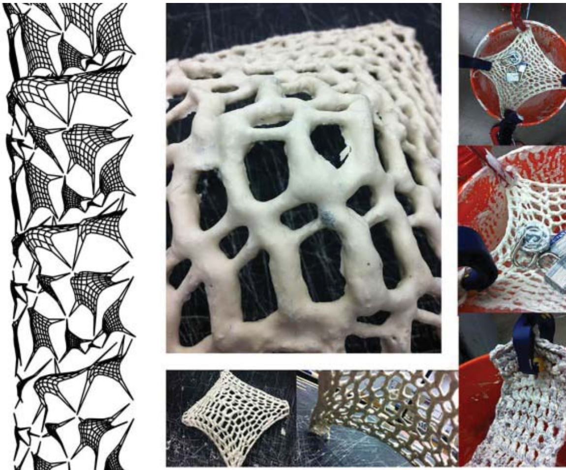
Figure 4: Soft material, Gaudi Catenary study. The “soft” panels are freeze into series of static panels and later used as skin component.
