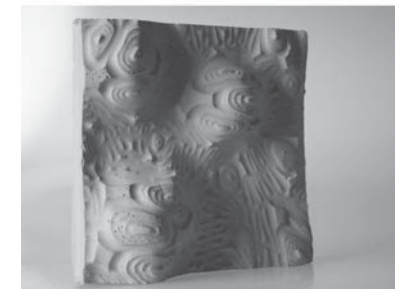
Figure 4 The CNC tool path generated through mathematical patterns and mapped directly onto a surface to produce ornamentation effects.
